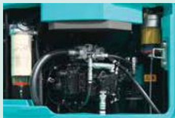
Fuel filter with built-in water-separator
