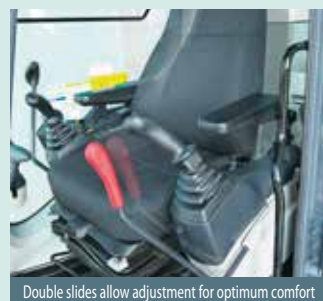
Double slides allow adjustment for optimum comfort
