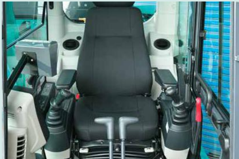
Seat suspension absorbs vibration
