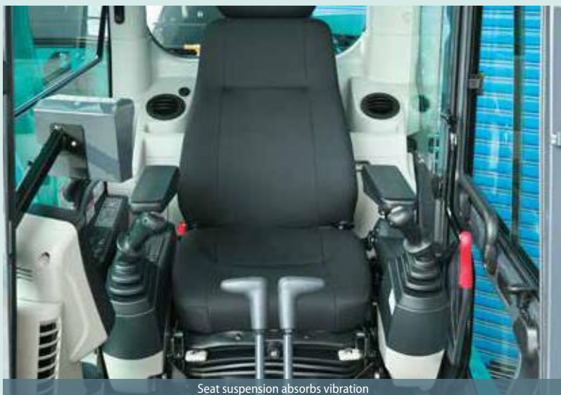
Seat suspension absorbs vibration
