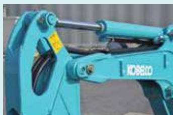
Bucket cylinder hoses sited within the arm
