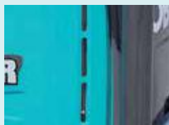
Fuel tank gauge
